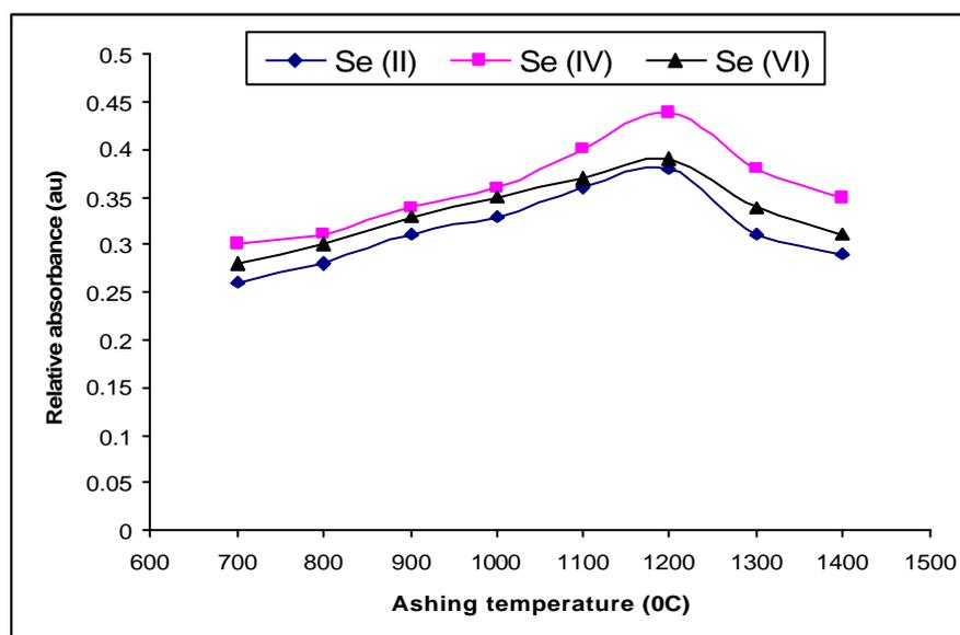
Fig. (2): Effect of the ashing temperature (atomization fixed at 2100 °C) on the absorption signals of 20 µg/L Se (II), Se (IV), and Se (VI), using Pd/magnesium nitrate as a chemical modifier.
