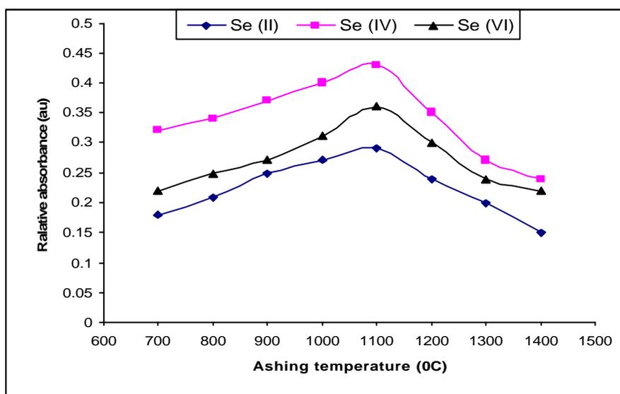
Fig. (1): Effect of the ashing temperature (atomization fixed at 2100 °C) on the absorption signals of 20 µg/L Se (II), Se (IV), and Se (VI), using nickel nitrate as a chemical modifier.
