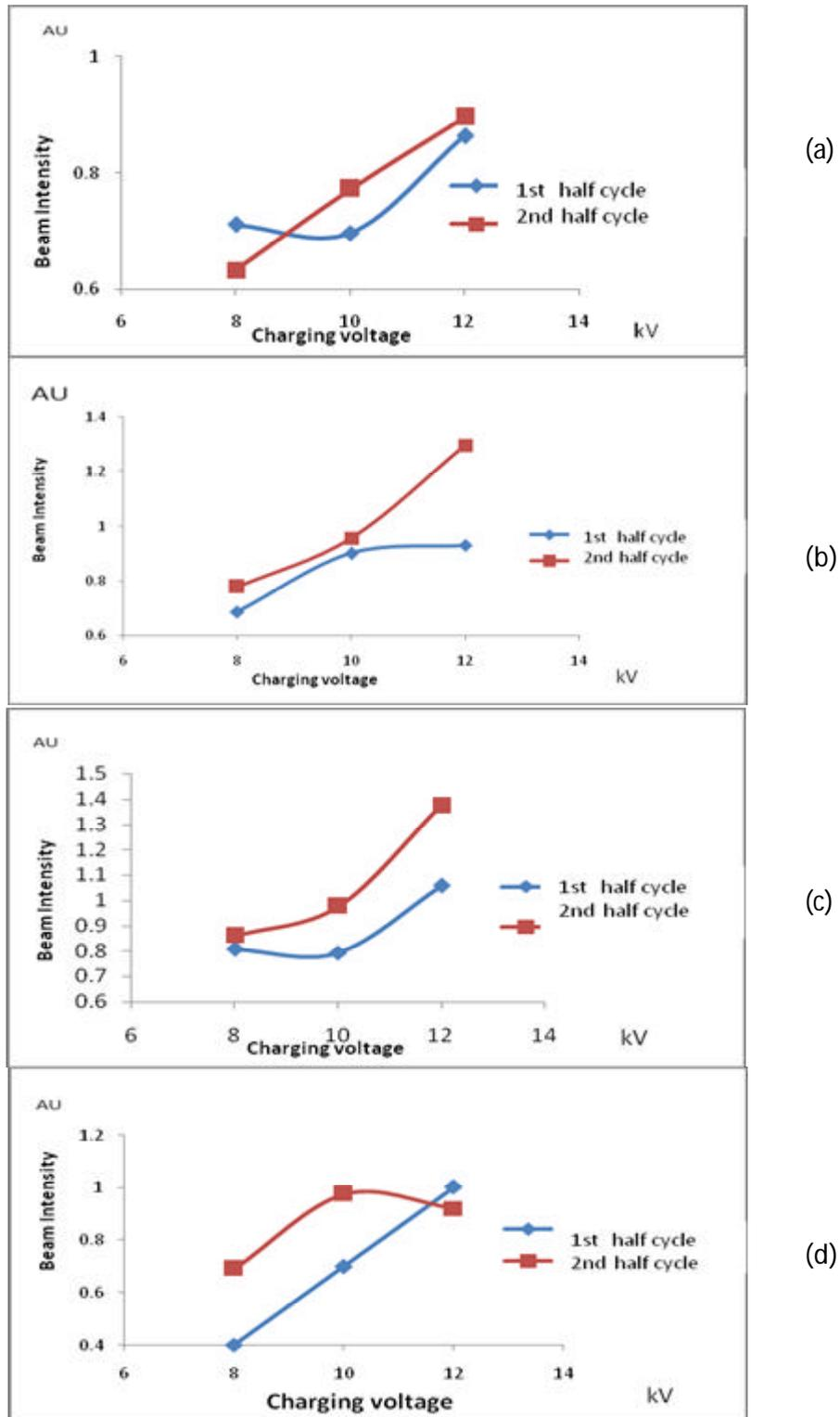
Fig.4 Variation of charged particle beams intensity with charging voltages at different argon filling pressures:
