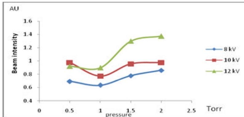
Fig.5 (b) Electron beams intensity vs. gas pressure at 8,10,12 kV (2<sup>nd</sup> half cycle).
