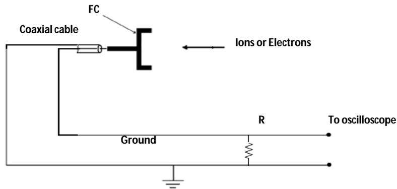
**Fig.2 Schematic diagram of the used Faraday cup**
