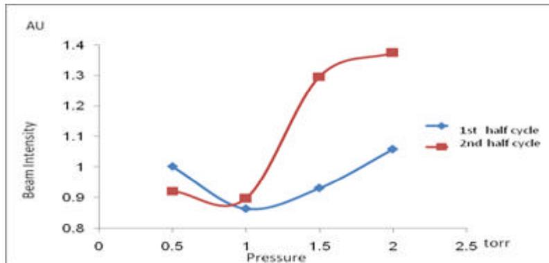
Fig.3 (c) variation of charged particle beams intensity with argon filling pressures at charging voltage 12 kV .
