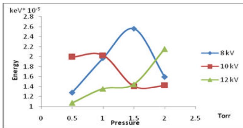
**Fig.6 (b) Variation of electron beams kinetic energy vs. filling pressure at 8, 10, 12 kV (2<sup>nd</sup> half cycle).**
