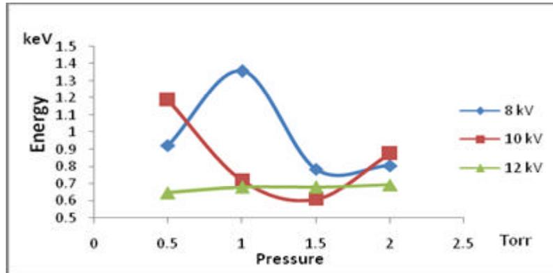
**Fig.6 (a) Variation of ion beams kinetic energy vs. filling pressure at 8, 10, 12 kV (1<sup>st</sup> half cycle).**
