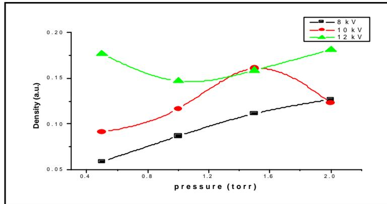
**Fig. 7 (a) Density of ion beams vs. filling gas pressure at 8, 10 and 12 kV (1<sup>st</sup> half cycle).**
