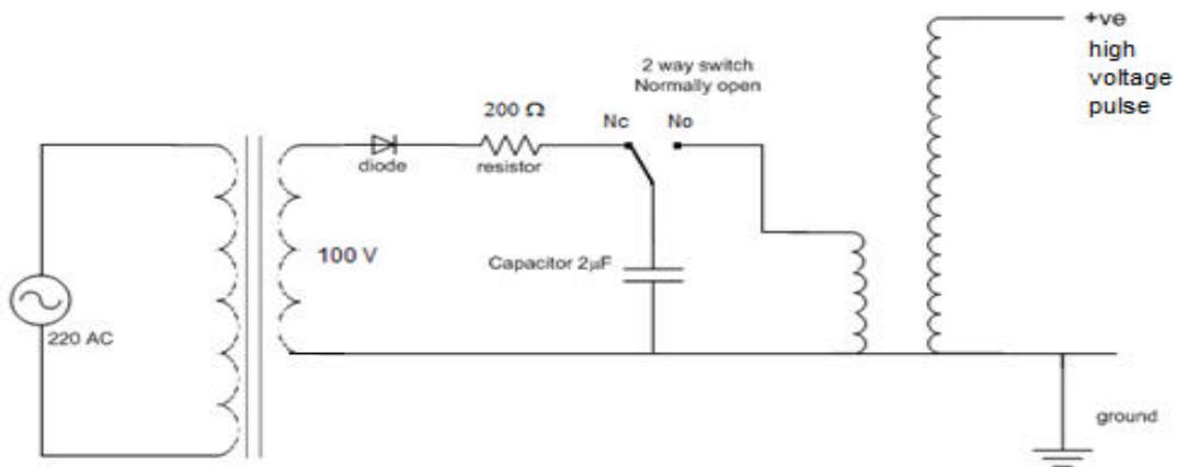
Fig.1 (c) The electric circuit of the triggering system
