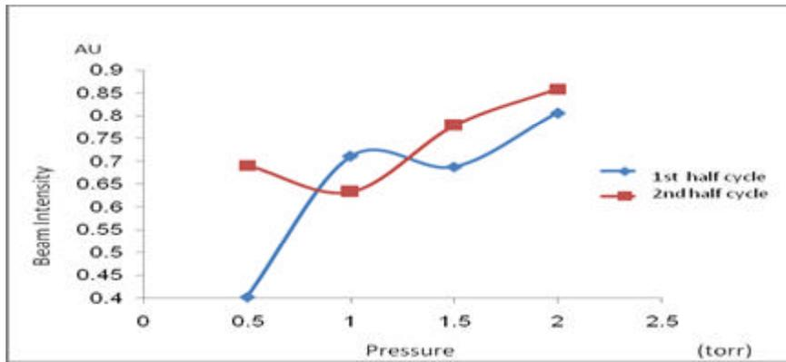
Fig.3 (a) variation of charged particle beams intensity with argon filling pressures at charging voltage 8 kV
