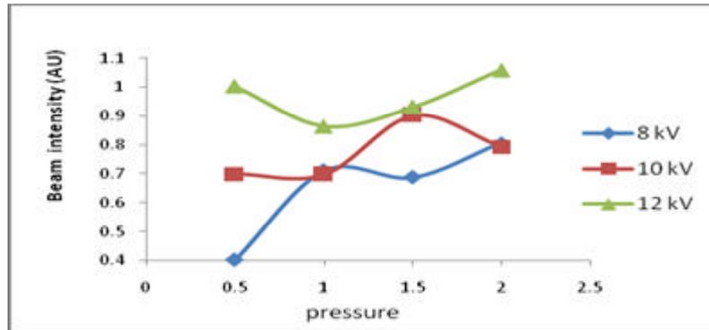
Fig.5 (a) Ion beams intensity vs. gas pressure at 8, 10, 12 kV (1<sup>st</sup> half cycle).
