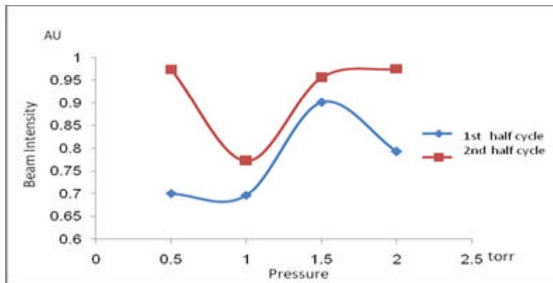
Fig.3 (b) variation of charged particle beams intensity with argon filling pressures at charging voltage 10kV
