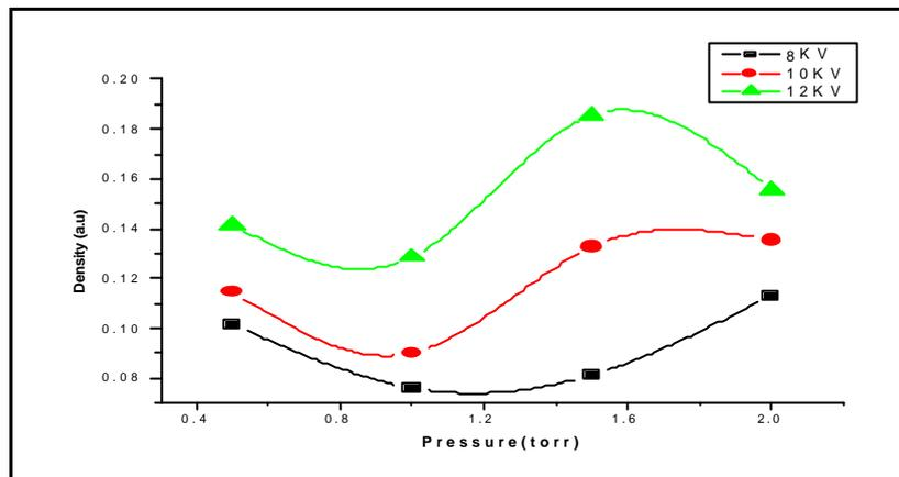
**Fig.7 (b) Density of electron beams vs. filling gas pressure at 8, 10 and 12 kV (2nd half cycle).**
