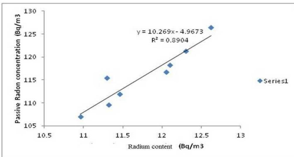
Fig. (4): Relation between the radium content and passive radon concentration.
