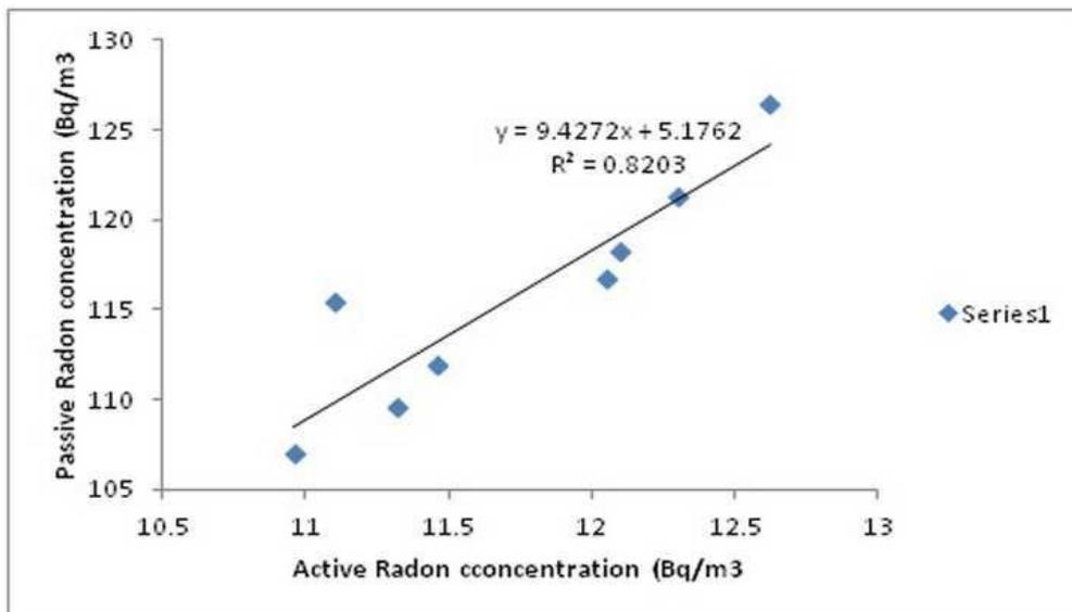
Fig. (5): Relation between active and passive radon concentration.
