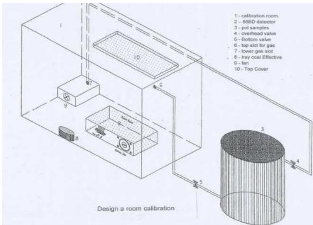
Fig. (2): Design room calibration to measure the temperature and relation humidity during radon measurement.
