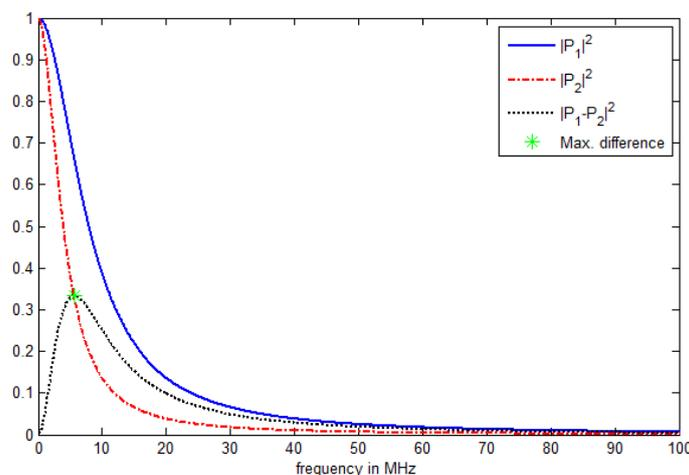
**Fig. (1):** Frequency magnitudes squares spectrums of  $P_1$  ( $\tau_1 = 20$  ns) and  $P_2$  ( $\tau_2 = 40$  ns), and their differences indicating the maximum difference of spectrums at 5.627 MHz.
