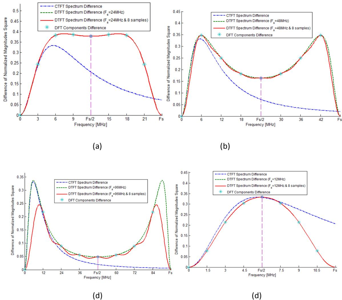
**Fig. (4):** Normalized differences of frequency magnitudes squares spectra using different fourier transforms at sampling rates of (a) 24, (b) 48, (c) 96, and (d) 12 MHz; for a window of 8 Samples.
