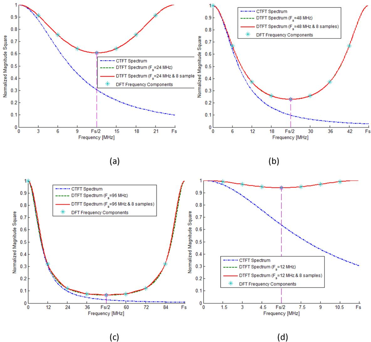
**Fig. (2):** Normalized spectra of frequency magnitudes squares for  $P_1$  ( $\tau_1 = 20$  ns) using different Fourier transforms at sampling rates of (a) 24, (b) 48, (c) 96, and (d) 12 MHz; for a window of 8 samples.
