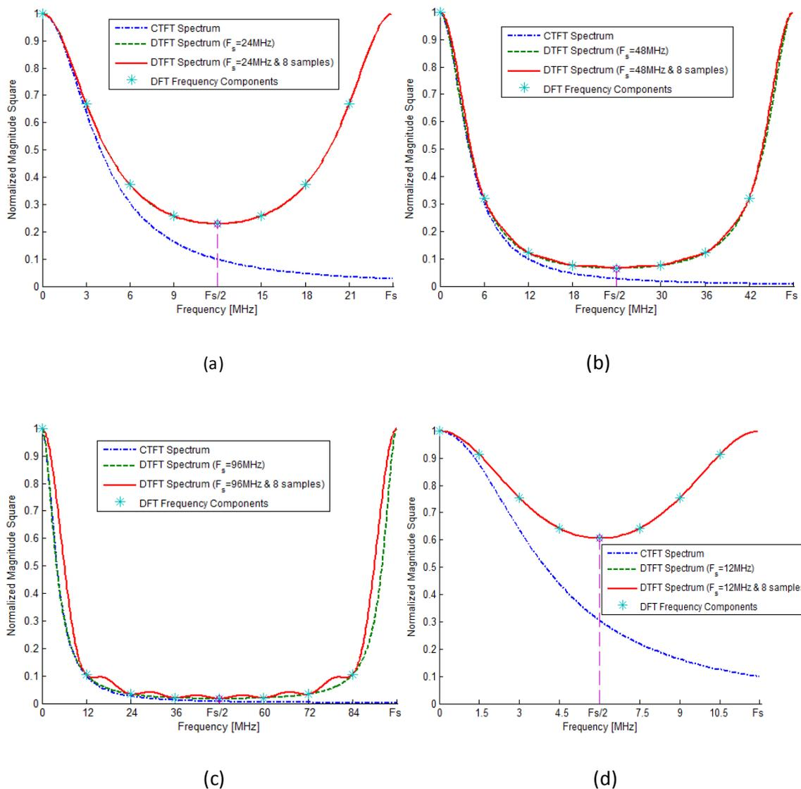
**Fig. (3):** Normalized Spectra of frequency magnitudes squares for  $p_2$  ( $\tau_2 = 40$  ns) using different Fourier transforms at sampling rates of (a) 24, (b) 48, (c) 96, and (d) 12 MHz; for a window of 8 samples.
