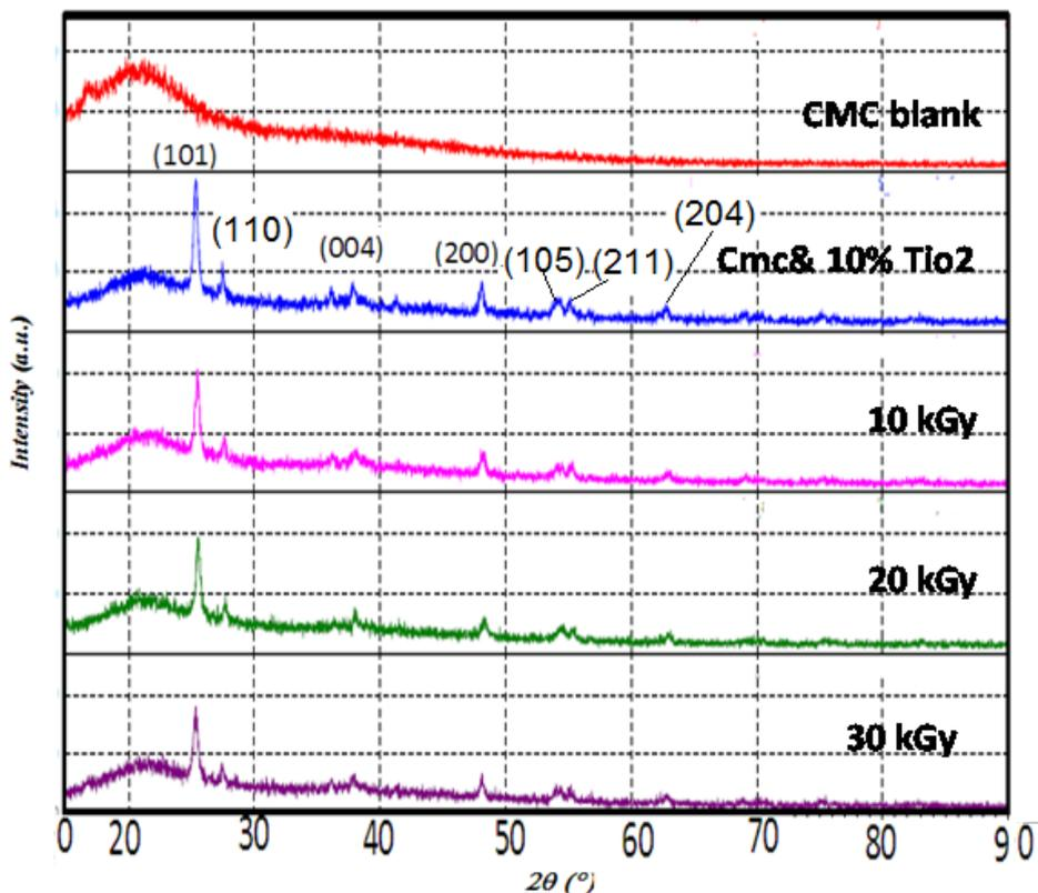
**Fig. (1):** XRD for the CMC, CMC/10% TiO<sub>2</sub> and irradiated CMC/TiO<sub>2</sub>(10%).
