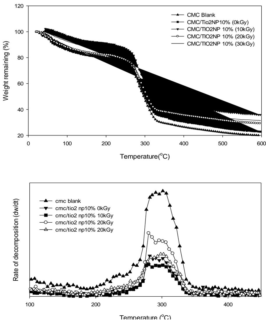
**Fig. (5):** TGA thermograms and the rate of thermal decomposition reaction of unirradiated CMC/10% TiO<sub>2</sub> and that exposed to various doses of gamma radiation.
