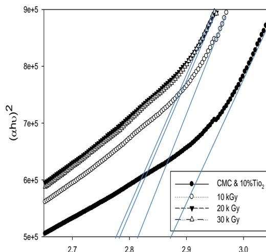
Fig. (4b): Energy band gap spectra for of CMC/10% TiO<sub>2</sub> exposed to various doses of gamma irradiation
