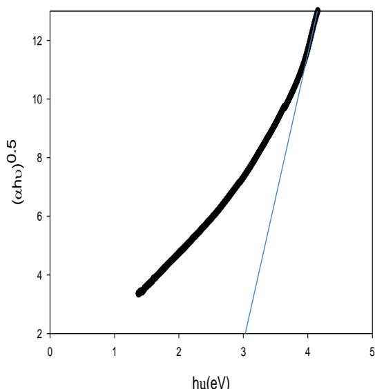
Fig. (4a) : Energy band gap spectra for CMC blank
