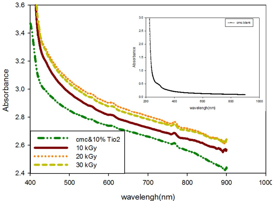
**Fig. (3):** Absorbance spectra of the CMC, CMC/10% TiO<sub>2</sub> and irradiated CMC/10% TiO<sub>2</sub>
