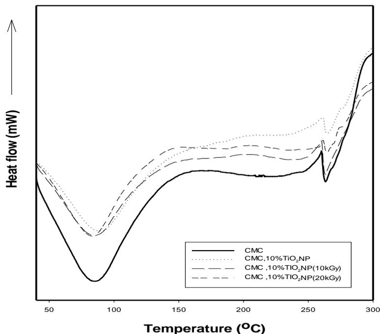
**Fig. (6):** DSC Thermograms of CMC/10% TiO<sub>2</sub> exposed to various doses of gamma radiation.
